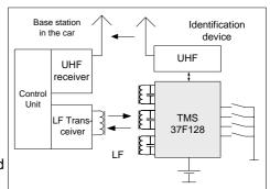
The embedded DST+ transponder offers a high level of security through its encryption, mutual authentication and after-theft diagnosis features; it operates without battery. The power management features in addition to battery charge/check a battery backup function which allows to operate all functions (including the microcontroller) with low or even no battery; the energy is generated from the LF field. The CRAID is available as flash (TMS37F128) and ROM (TMS37C128) version.
